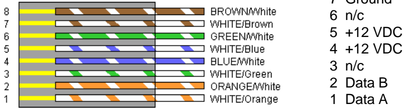
RJ45 Plug Colour Code Contact Side - Tab is on Back
